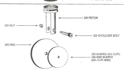
\*\*\*For Model AH-15-GL the four parts shown below line are replaced with the 300-01 Aluminum Piston and the 5/16-18 x 1-1/2" Screw
